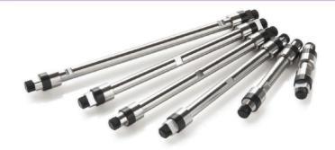
Orochem Technologies provides a wide range of traditional liquid chromatography columns. These columns are packed in various modes, such as reversed phase, normal phase, and ion exchange. The particle size ranges from 1.7-300 µm, pore size ranges from 90-300 Å, and various dimensions.
