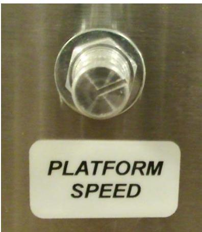
**Figure 6: Valve for Controlling the Platform Speed**
