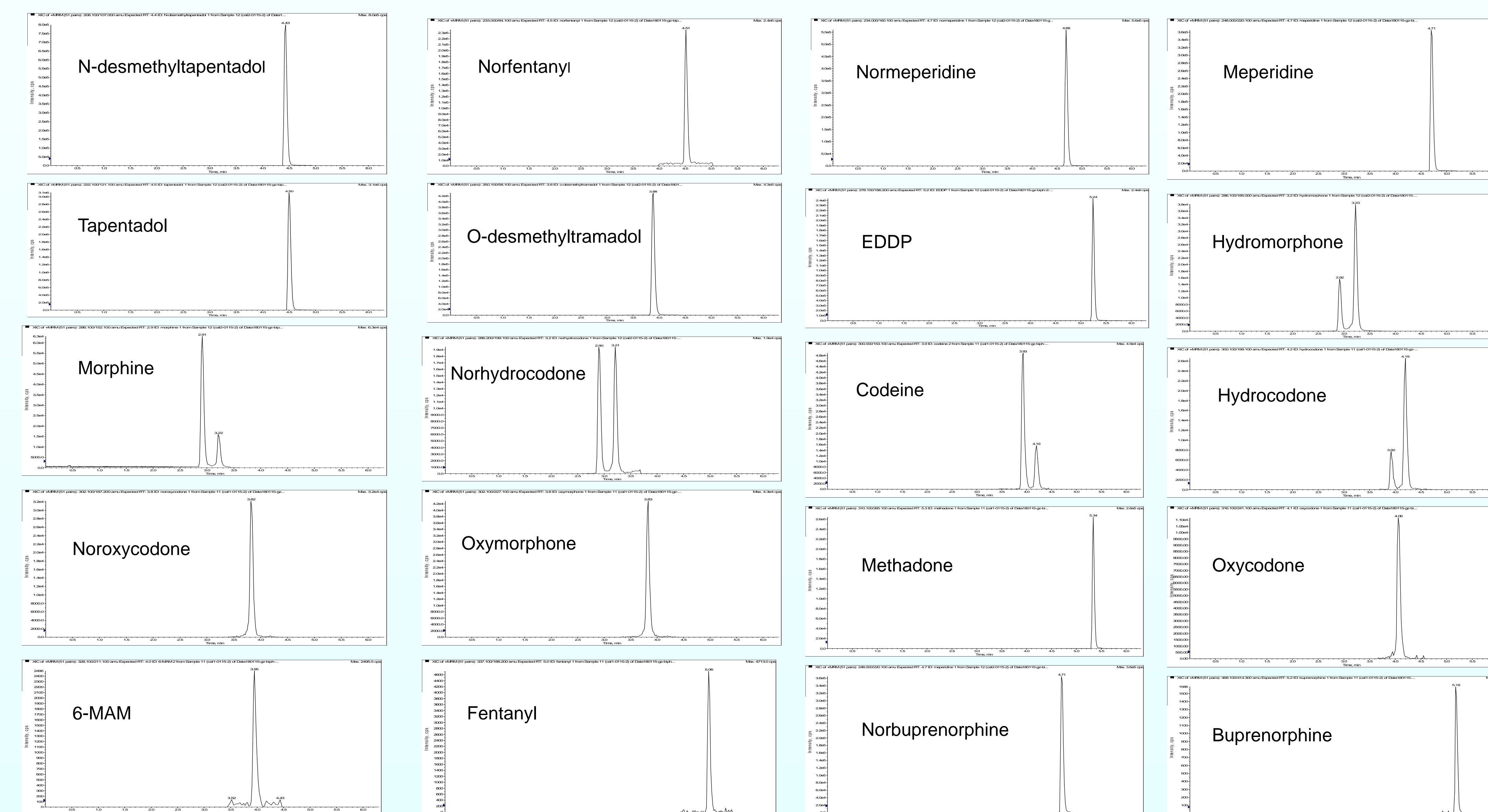
Mass chromatograms of SPE extracts from opiate drugs and metabolites fortified urine
